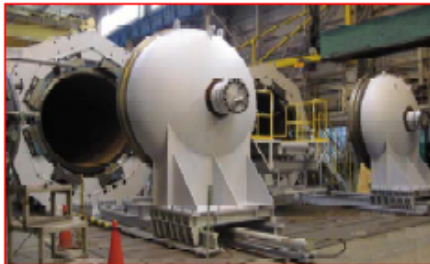
Testing of DAVINCH Chambers for China
