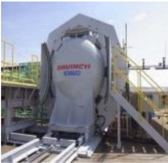
Controlled Detonation Chamber
