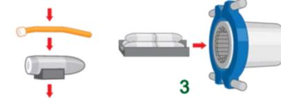
Linear-shaped charges are attached along the munition body and the item is placed in the munition holder (up to 6 pack).
