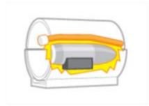
Operators remotely detonate the linear shaped charges to access the munition body and destroy explosives.
