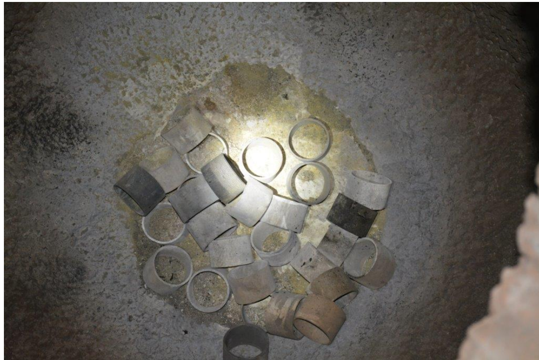
Inside of Detonation chamber after Test 2 (Pipe sections added for weight)
