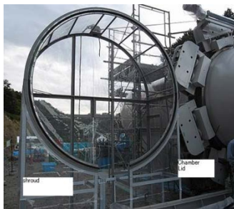
Shroud (Keep the dust in it when the Lid is opened)
