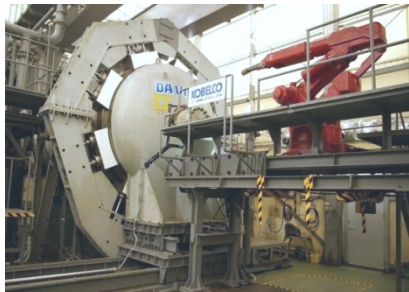
The moving deck and robotic (Transport the munition and hang it on the hook)
