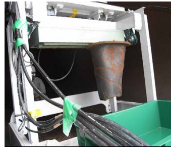
Magnet lifter (Remove the fragment after detonation)
